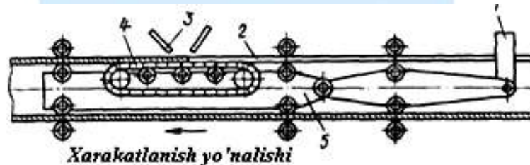
1-rasm. Quvur tashqi chokini payvandlash jihozi
