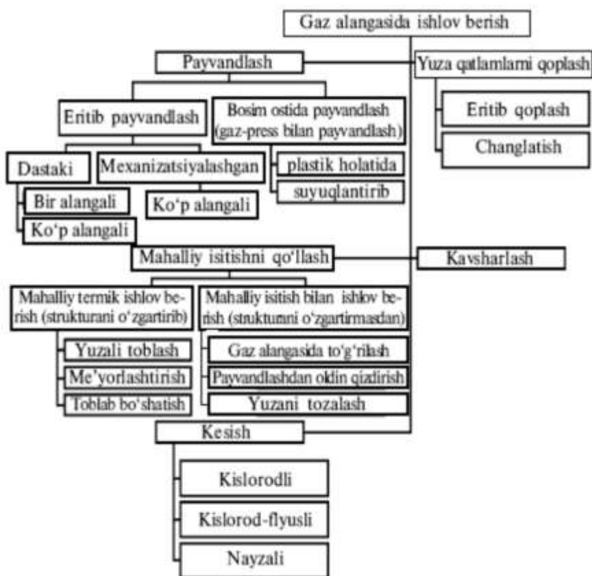
1-rasm. Gaz alangasida ishlov berishning strukturaviy sxemasi
