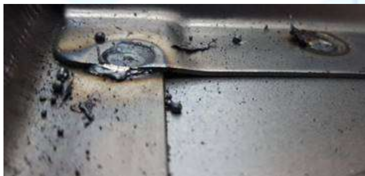
2-Rasm. Kontaktli payvandlash paytida sochramalar paydo bo'lgandan keyin panelning holati
