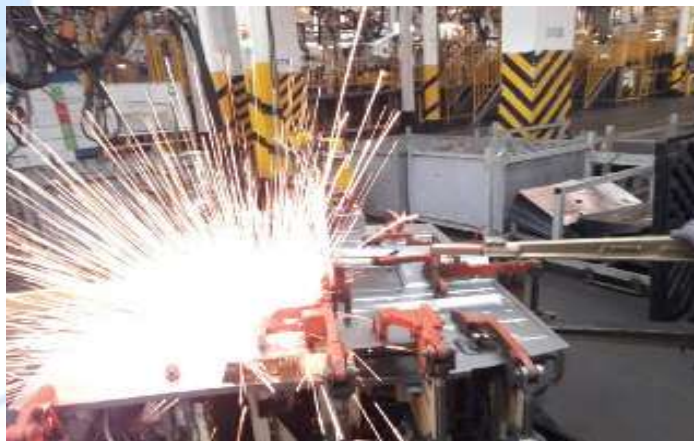
1-Rasm. Nuqtali kontaktli payvandlash jarayonida sochramalar paydo bo'lishiga misol
