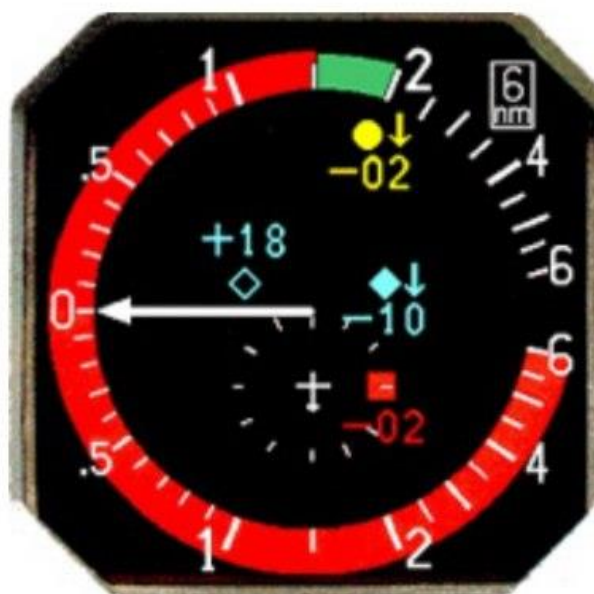
Picture 1: Example of ACAS II traffic display, indicating a "Climb" RA with a target vertical speed of 1500 ft/min.
