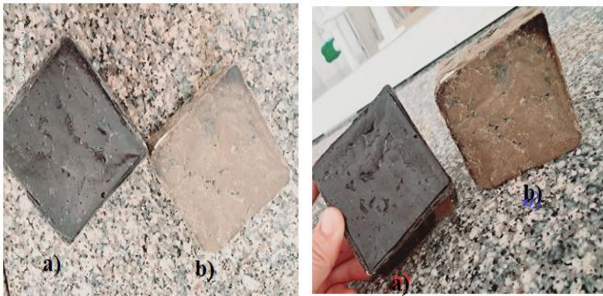
1-rasm. Chiqindi holdagi plastmassalardan olingan bruschatkalar a) qora rangli b) sariq rangli
