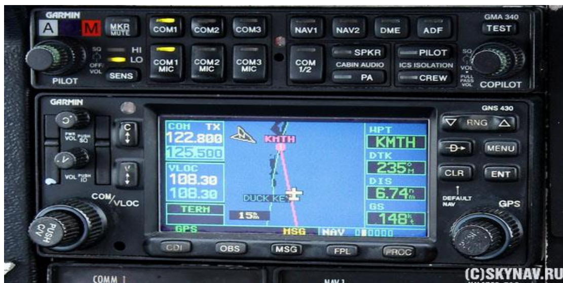
Figure 3. Garmin GNS-430. One of the most common aviation GPS receivers
