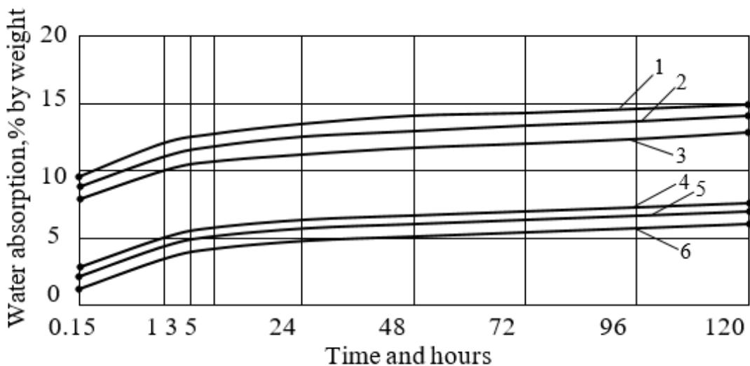
Rice. 1. Dependence of water absorption of concrete on time and type of filler.
