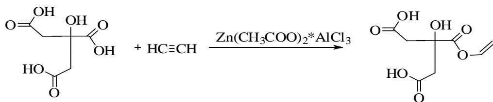
The monovinyl ether formed by the acid reacts with acetylene in the presence of a catalyst to form divinyl ether.
