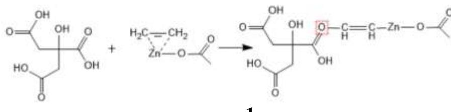
The formed citric acid undergoes the compound of mono vinyl ether with aceto-zinc  $\beta$ -elimination, then its mono vinyl ether forms 2.
