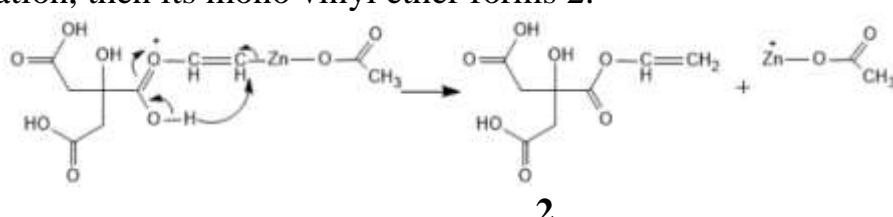
In the same order, the second and third carboxyl groups are also vinylized and then divinyl (2-schema) and trivinyl ethers of citric acid are formed (3-schema). The process, of course, takes place through the formation of the complex of mono vinyl with aceto-zinc and the complex of divinyl acid with aceto-zinc.
