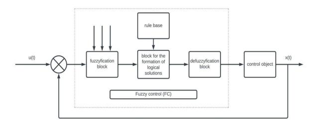
Figure 1. Functional scheme of the intelligent control system based on fuzzy logic. Oil is a liquid substance consisting of a complex mixture of hydrocarbons. Oil with a temperature of around 10 °C is transferred to the heat exchanger through a pipe. The imported raw material is introduced into the heat exchanger device. Gasoline, the light fraction of the produced oil, is used as a heating agent.
