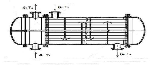
Figure 2. A view of a shell-and-tube heat exchanger.
