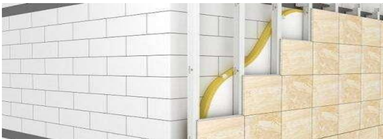
Fig. 3 Fasadbop marble tiles
